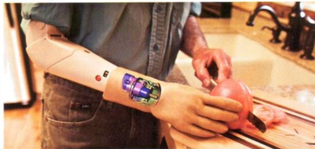
InHand Wrist Rotator. Photograph courtesy of Motion Control.
