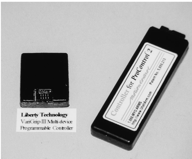
Figure 21. Size comparison between the VariGrip III and ProControl II extrinsic processors. Note the ProControl II is available as an intrinsic processor within the Motion Control Hand.
