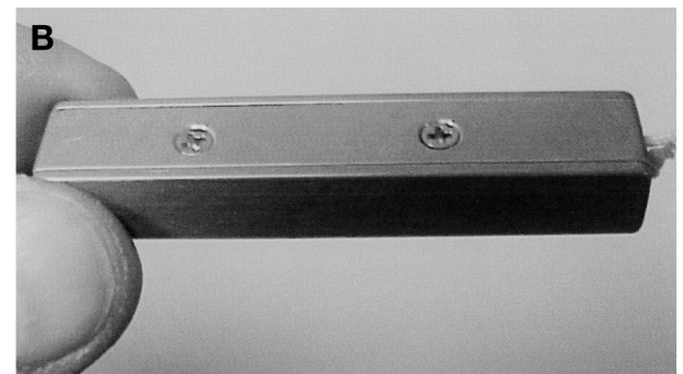
Figure 14. A: Linear Transducer from Liberating Technologies (courtesy of Liberating Technologies, Inc.). B: Direct relationship of force to elbow positioning can be found in the Motion Control ServoPro force sensor (Image courtesy of Motion Control, Inc.).
