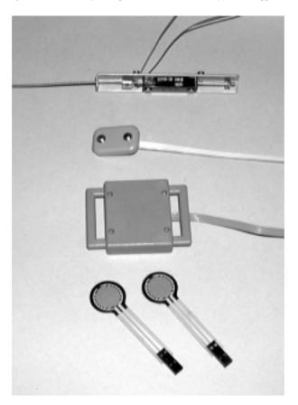
Fig. 4. Input Devices (from top) Linear Transducer - servo, myo-electrode, harness switch, force sensing reducer - touch pads.
