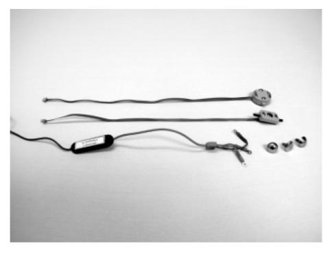
Fig. 5. Comparison of Otto Bock and Motion Control Style electrodes.
