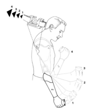
Fig. 3. Direct relationship of force to elbow positioning can be found in the Motion Control Servo Pro Force Sensor. (courtesy of Motion Control, Inc).
