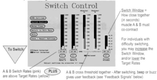
Fig. 11. Pro Control II Switch Control Window accessed for adjustment of co contraction switching between wrist and hand function. (courtesy of Motion Control, Inc).
