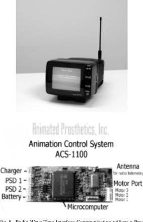
Fig. 8. Radio Wave Type Interface Communication utilizes a Prosthesis Configuration Unit (PCU) – (Top) to program the processor (Bottom) (courtesy of Animated Prosthetics, Inc).
