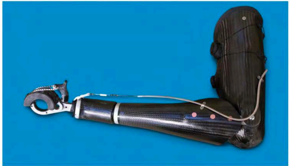
MacJulian “Mac” Lang, CPO, FAAOP, and technician Cullen Hays designed an above-elbow body-powered prosthesis with a quick-release feature to allow Anderson to disengage quickly.
